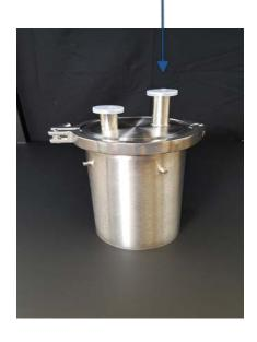
The Shorter KF-25 stub ALWAYS connects to the VACUUM Pump
