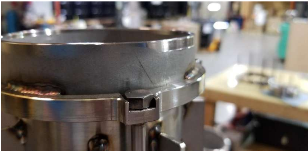
Fig 11. Roller rods are pinned at the bottom end of the baskets by the machined grooves that prevent them from spinning.
