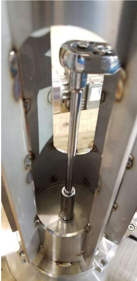
Fig 10. Reaching the drive shaft bolt
