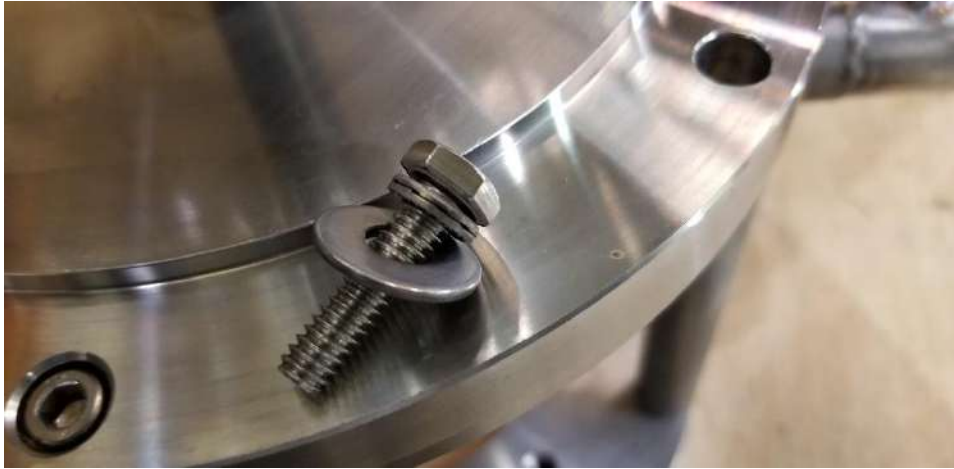
Fig 9. Drive shaft bolt setup. Note that the “Nord” lock washer is a two-piece locking washer and won’t perform correctly if one half is lost.
